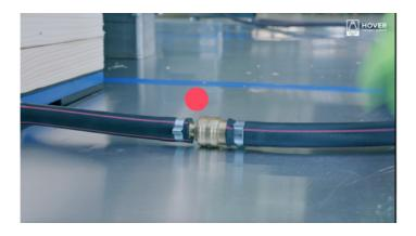
Connect the air interconnect hoses to the air control unit and make sure that the colour code is matching.
