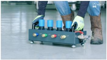
Take the air interconnect hoses out of storage or the transport case and lay them (with the correct colour) next to the air caster assemblies.
